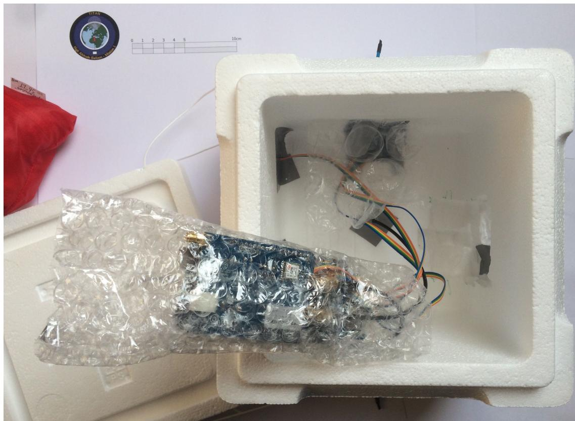
Figure 9: Payload box seen from top with open hatch, flight computer already wrapped in goffered plastic packing film.
