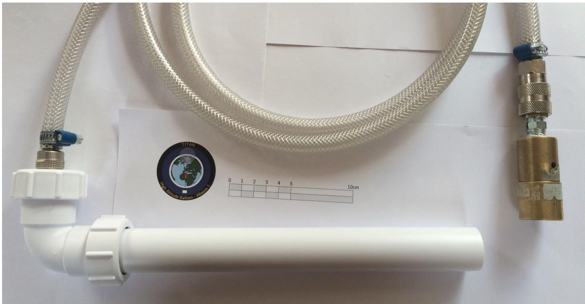
Figure 14: Filling tube with an outer diameter of 30 mm with hose and extra weight connected.
