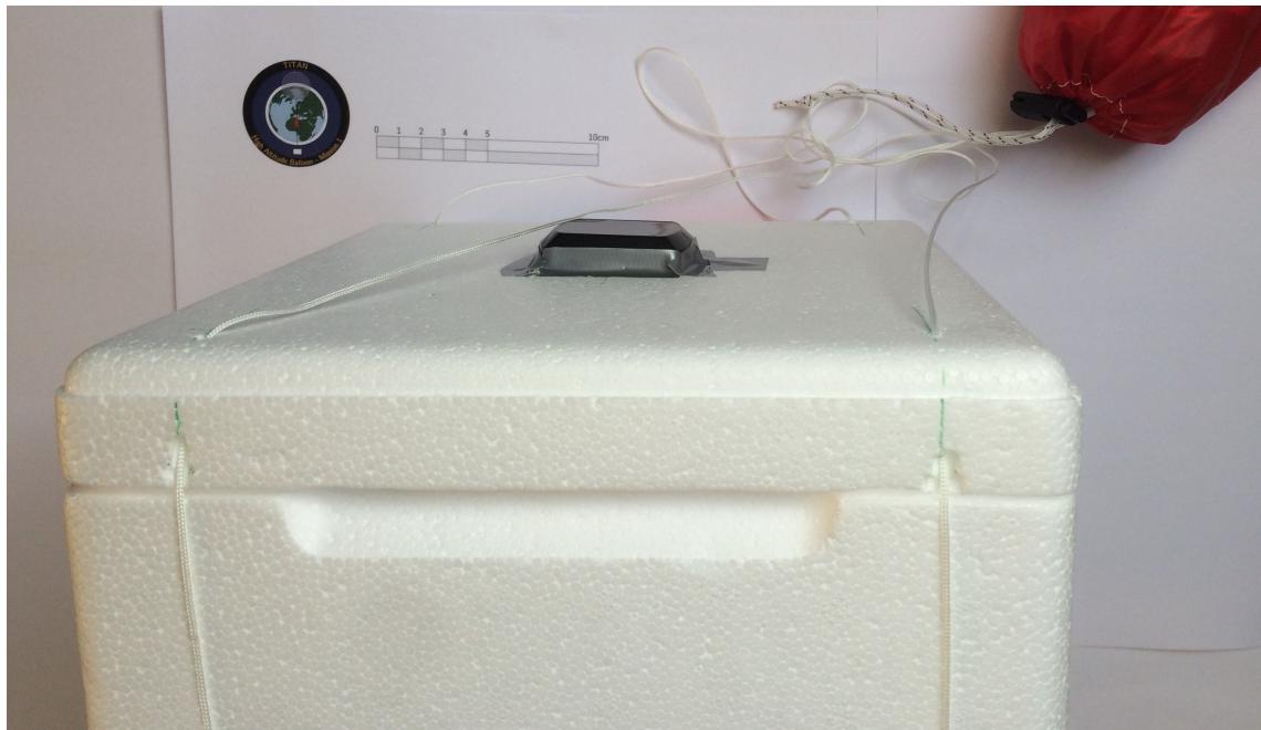
Figure 10: Closed payload box, the antenna on top is visible and the routing of the lines through the hatch.
